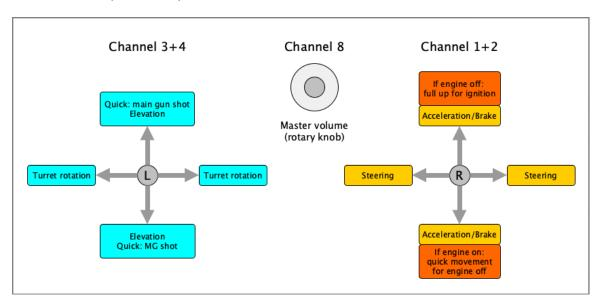
The ignition and acceleration/brake control is made by channel 1 (brown wire). After power up the engine doesn't run and the vehicle cannot be moved. To start the engine the throttle control must be moved to the upper most position and hold until the ignition sequence starts (see image below). Wait until the ignition sequence is finished and the idle sound is played. Now the vehicle is operational.
