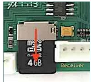
**Never drag the card in a direction other than the one shown! This can lead to permanent mechanical damage to the card holder and thus to destruction of the electronics!**
