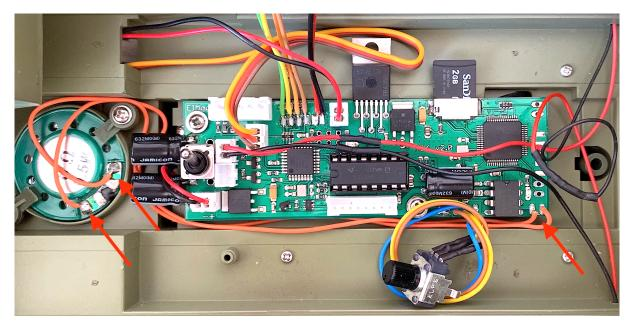
Connect the 8-pin tower plug to connector 10 and the 2-pin muzzle flash plug to connector 7. The muzzle flash plug can be aligned in any way as both contacts on the circuit board are connected together.
