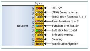
Depending on the used RC it may be necessary to change the order of the channels or to inverse the servo travel. Please read the manual of your RC gear for details. The signal of channels, that remains unused must not be connected.
