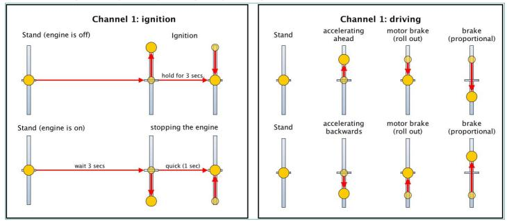
To switch off the motor, proceed as follows: stop the vehicle for at least three seconds. After that the throttle stick must be put to the bottom and released back quickly to the center position. This procedure may not last longer than one second. Is the motor restarted after just a short time, a shorter start up sequence (warm start) is played. The time of cooling down the engine may also be configured by the software.
